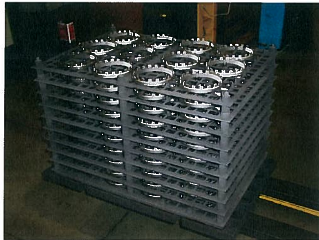
Fig. 4: CFC-fixturing for internal ring gears
